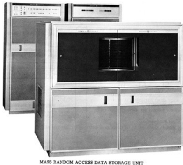
Figure A.2 The data storage unit with its platters
